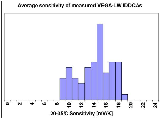
Figure 2-3: 20°C-35°C average Sensitivity over 70 IDDCAs, 75K, no FOV correction
