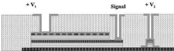
Figure 4.1: dual band QWIP structure
