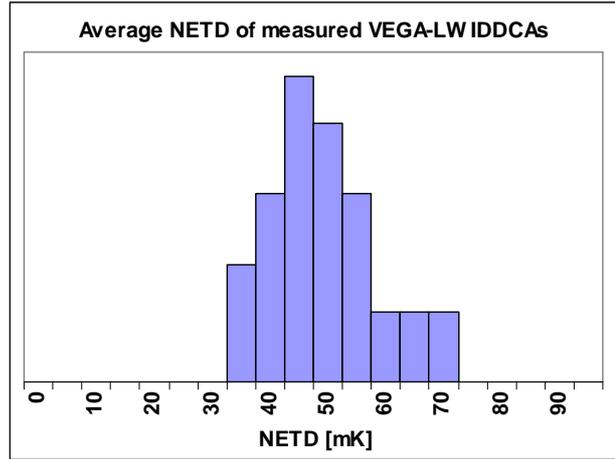
Figure 2-4: NETD over 70 IDDCAs, 75K, with FOV correction
